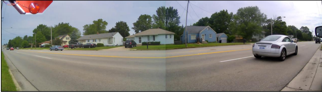
Shown above is a view from the stop-arm camera mounted forward of the stop-arm on a bus. Note that the stop arm is partially in the view when open but not obstructing license plate capture
