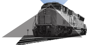
A forward-facing camera captures conditions in front of the locomotive and two in-cab dome cameras that monitor all activity in the cab.
